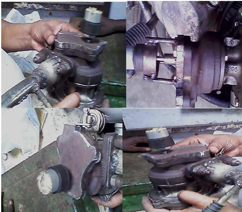
Fig.4.Fabricated model Turbo charger connected with exhaust pipe
